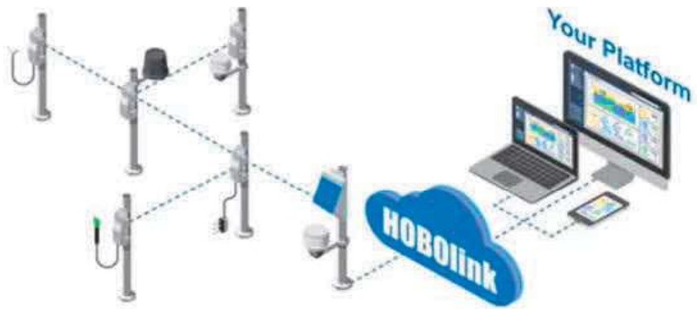
Figure 22 All Sensor Data is Collected to a Data Logger Module
